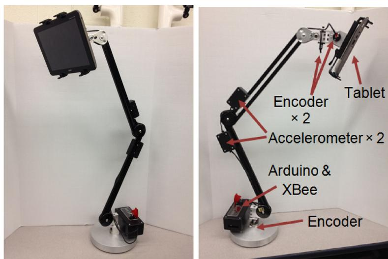
The master arm controller uses 5 sensors to measure the **5 degrees of freedom of the master arm**. With an encoder in the base and two accelerometers on the arm, the 3D position of the tablet computer can be calculated. Two encoders measure the pan and tilt orientation of the tablet. The tablet displays a **3D visualization of the slave arm** as well as **video from the slave**.
