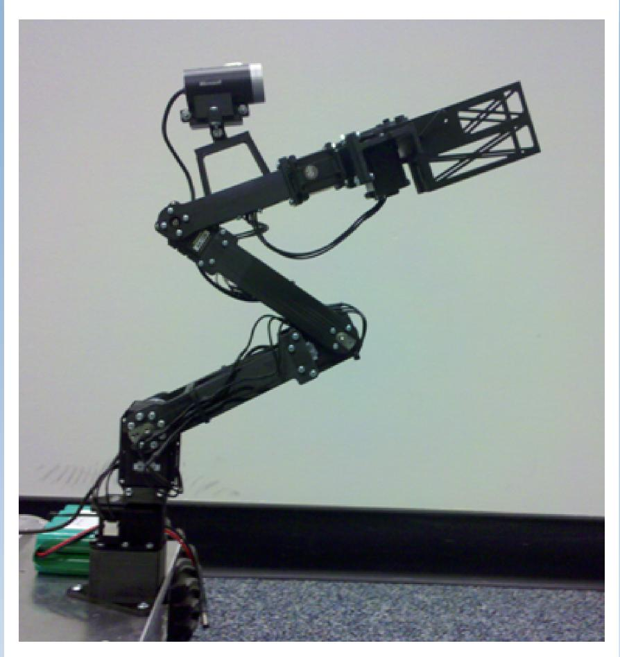
The master controller only specifies the desired camera position and orientation, so **any slave arm with a suitable workspace could be controlled** with this input system by calculating the inverse kinematics. One arm used for demonstration of this control system is shown above. A different arm is shown in the photo in the box to the right.
